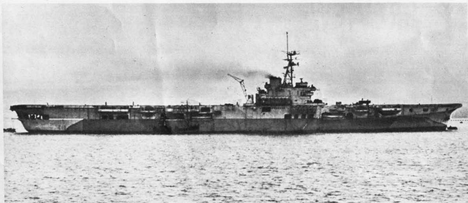
Colossus Class , new British CVL, is 695 feet long, displaces 14,000 tons. Although this is a new size for British carriers, the Colossus
